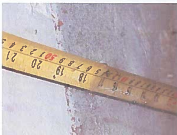
Day 1: Water level at one end 445 mm
